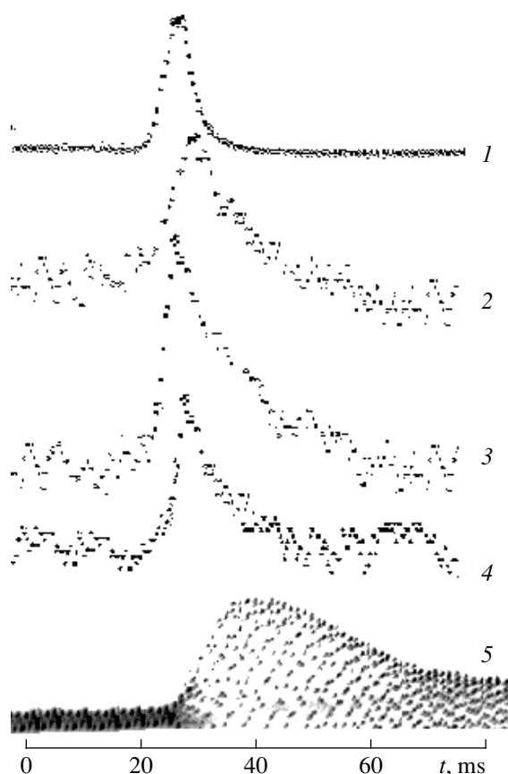
Fig. 5. Kinetics of luminescence at \lambda = (1) 306 nm, (2) 823 nm, (3) 846 nm, (4) 852 nm, and (5) 1.41 \mu\text{m} ( T = 300 K, P = 100 Torr, spark initiation).
